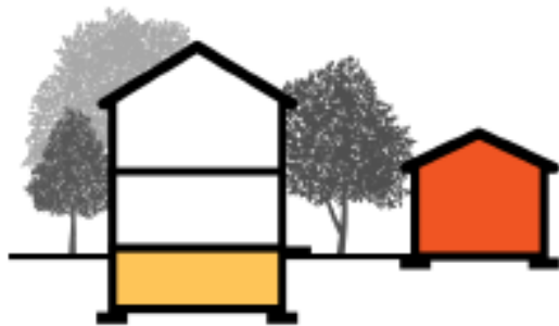
Figure 9 - Cross-section of 1 Interior ARU and 1 Detached ARU
