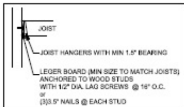
USING JOIST HANGERS CARRY JOISTS
