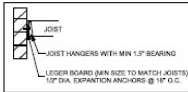
USING JOIST HANGERS CARRY JOISTS
