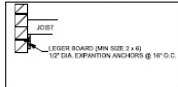
USING LEDGER BOARD TO SUPPORT JOISTS
