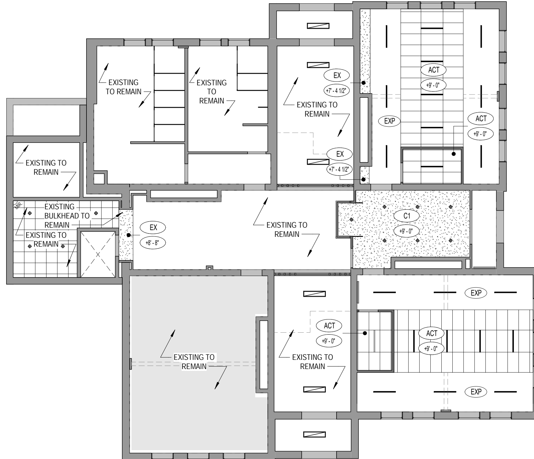
MAIN FLOOR REFLECTED CEILING PLAN
