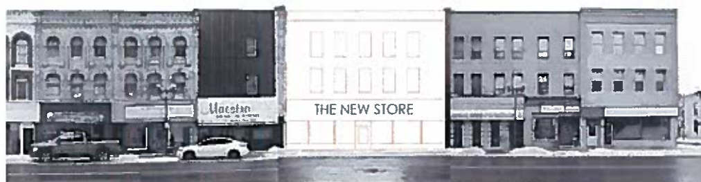
Plate 14: Sketch showing the recommended façade composition for new infill
