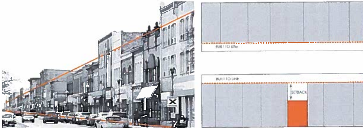
Plate 4: The setback of properties along Talbot Street forms a consistent street wall. This should be maintained as in the top right illustration. The bottom right scenario should be avoided
